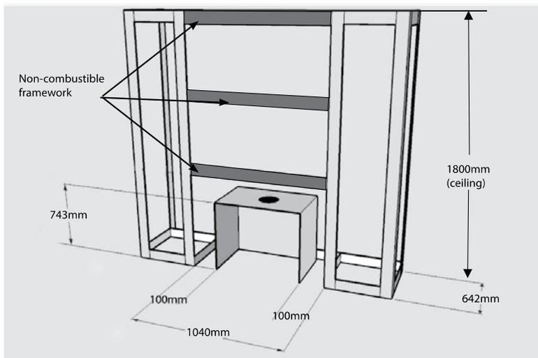
**IMPORTANT:** Non-combustible sheeting of a minimum thickness of 9mm must be used on the front face of the enclosure.
