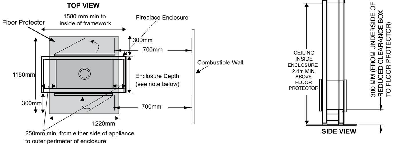
NOTE: Enclosure depth will depend on the the finished wall thickness on each side of the enclosure - see installation manual for details.
